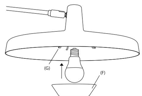
6. (E) To insert the light bulb, release the undershade (F) by pressing three undershade brackets (G) inwards.
