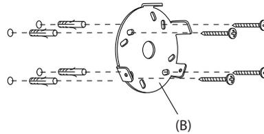
2. (E) Mount the wall mounting to the wall with four appropriate screws and plugs. Always use correct screws and plugs for the mounting surface.
