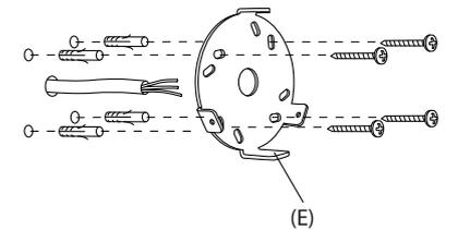
3. (E) Position the wall mounting making sure the metal handle (E) is covering the hole on the lamp body. Mount it with four appropriate screws and plugs. Always use correct screws and plugs for the mounting surface.
