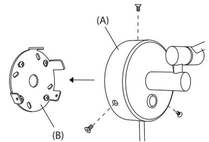
3. (E) Attach the lamp body back to the wall mounting.
