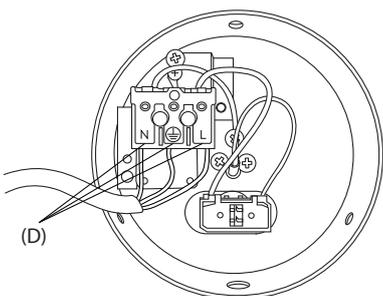
4. (E) Connect the electrical cord with the terminal strip.
