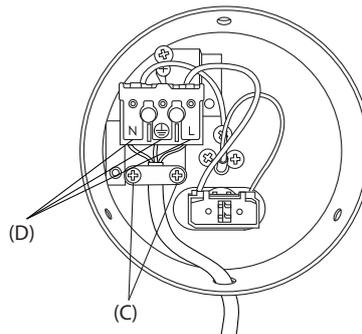
2. (E) Unscrew the two screws (C) from the back of the lamp housing. Press N, ⊕, L tabs (D) on terminal strip to pull the cord out.
