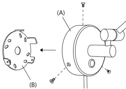
1. (E) Remove the wall mounting (B) by unscrewing three screws from the lamp body (A).
