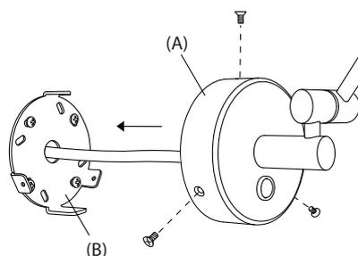
5. (E) Attach the lamp body back to the wall mounting.
